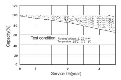
• Figure 2-7 Floating charge service life characteristic curve---24Ah and above batteries
